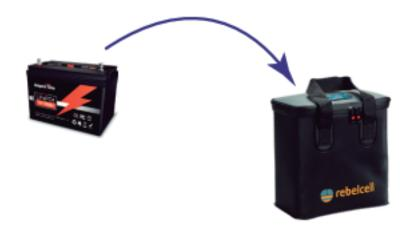
Do not to transport the battery with other elements in the same package as liquids or metal parts
